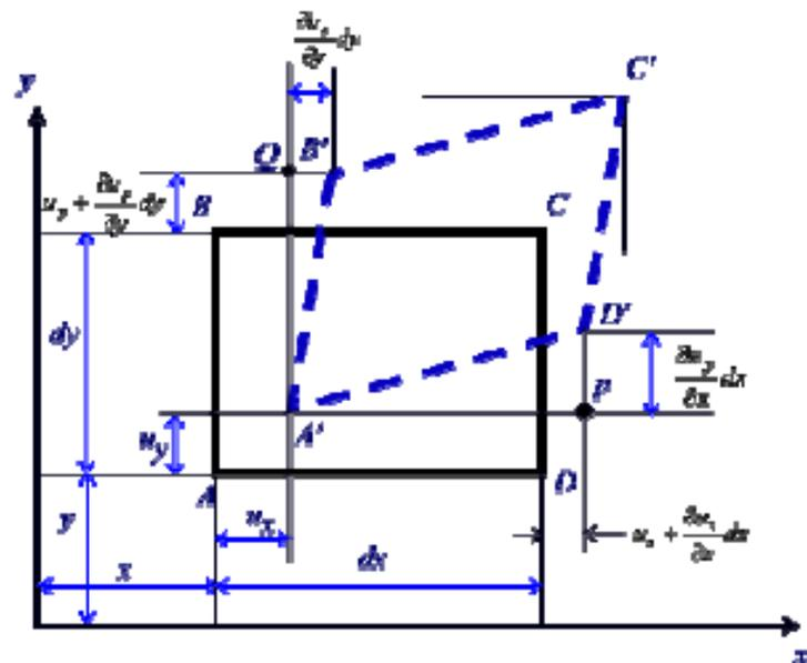
$$u_{xx} = \frac{A'D' - AD}{AD} \cong \frac{A'P - AD}{AD} = \frac{dx + \frac{\partial u_x}{\partial x} dx - dx}{dx} = \frac{\partial u_x}{\partial x}$$
